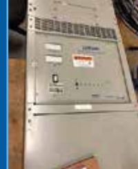
LORAIN FLOTROL RECTIFIER POWER SUPPLY
